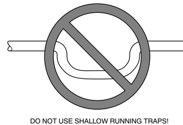
Fig. 13 – Insufficient Condensate Trap
