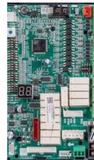
INDOOR AHU CONTROL BOARD
