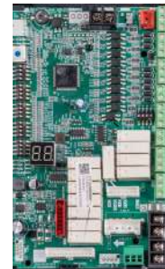
INDOOR AHU CONTROL BOARD
