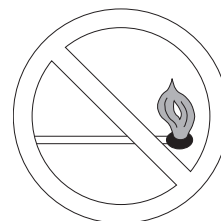
Fig. 3 – Do Not Light Burner with Match
