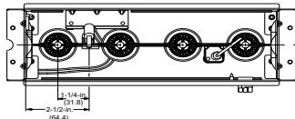
**Fig. 68 – Igniter Position - Top View**
