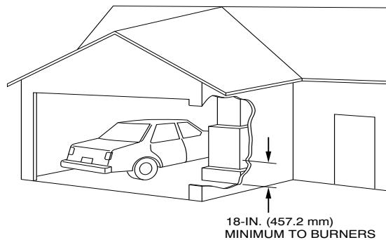
Fig. 5 – Installation in a Garage A93044
