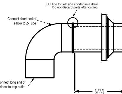
**Fig. 17 – Modify Rubber Drain Elbow Horizontal Orientation**
