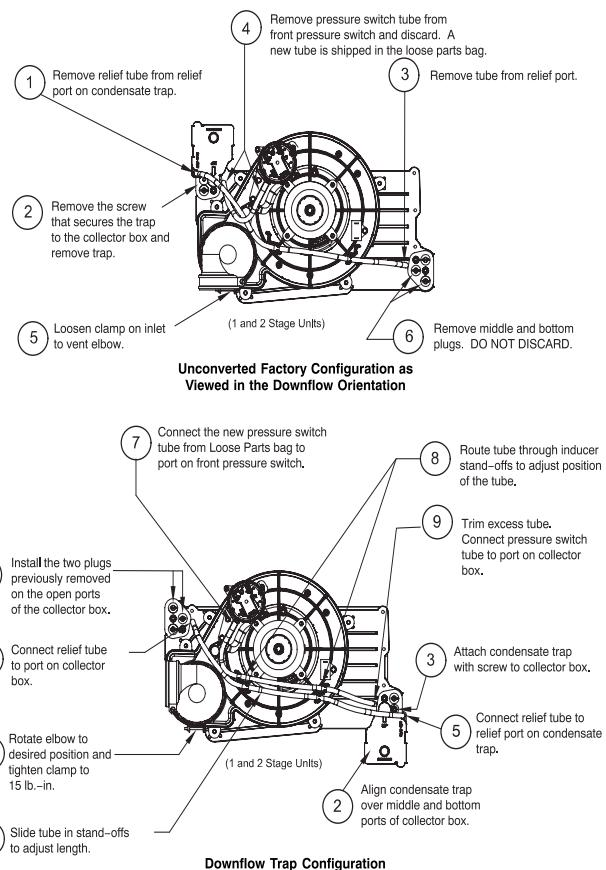
**Fig. 9 – Downflow Trap Configuration**
