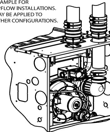
**Fig. 44 – Sample Inlet Air Pipe Connection for Polypropylene Venting Systems** A12220
