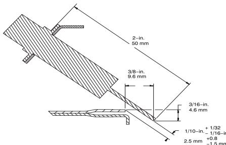
**Fig. 69 – Igniter Position - Side View**
