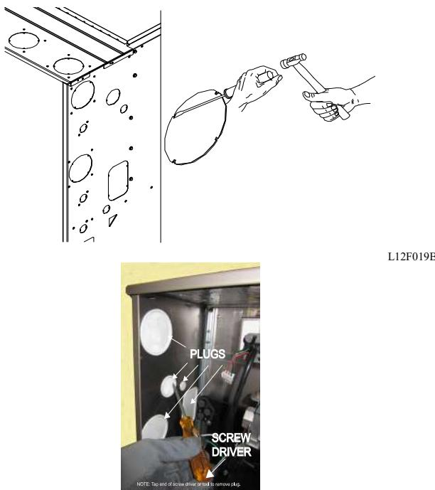
**NOTE:** Locate the plug that needs to be removed. Using a screw driver or tool, place end against rim on plug. Tap on the butt end of screwdriver or other tool to remove plug.
