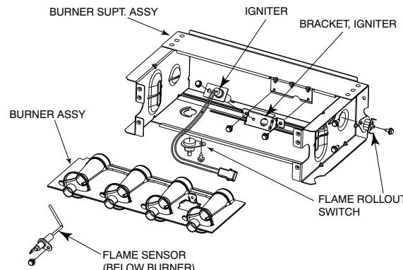
**Fig. 67 – Burner Assembly**
