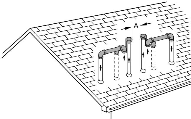
**Fig. 47 – Pipe Vent and Combustion** A96128
