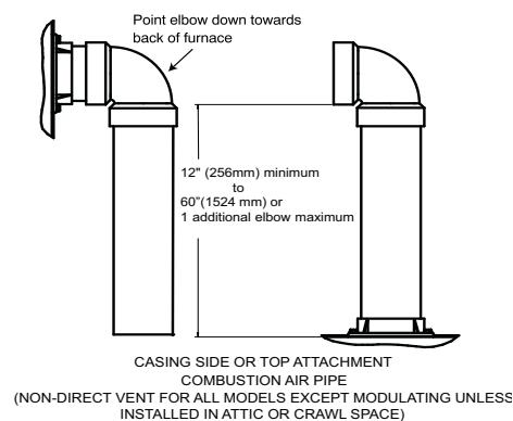
**Fig. 45 – Combustion Air Pipe Attachment** A13406
