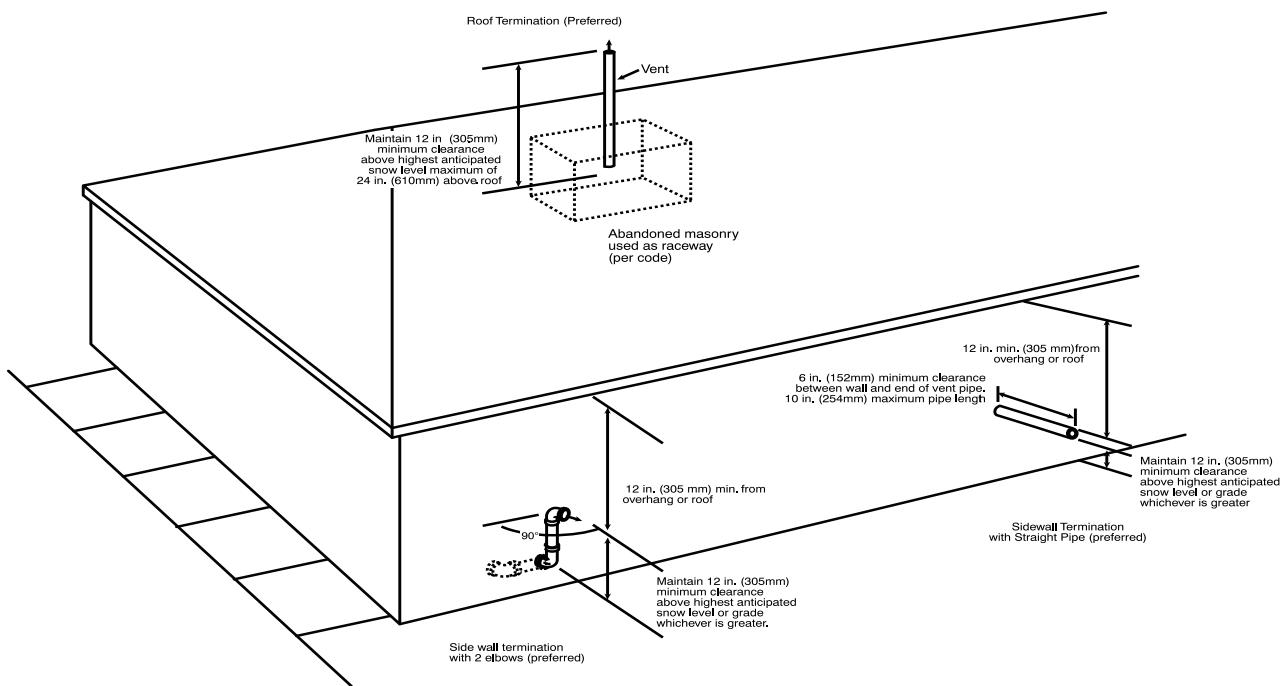
Fig. 40 – Vent Pipe Termination for Non-Direct Vent and Ventilated Combustion Air System
