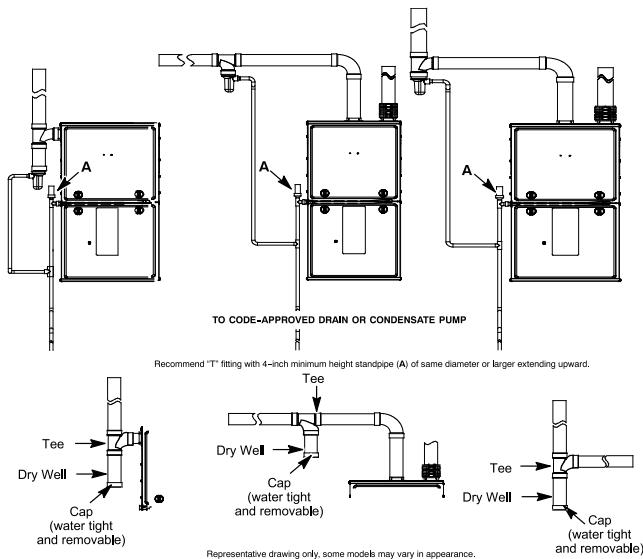
Fig. 50 – Recommended Combustion Air Inlet Moisture Trap A170122A
