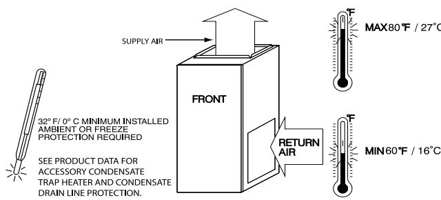
Fig. 3 – Freeze Protection and Return Air Temperature A150573
