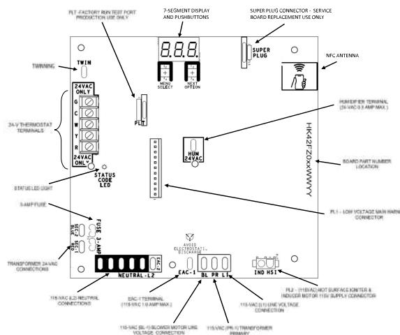
Fig. 37 – Example of Single Stage Furnace Control
