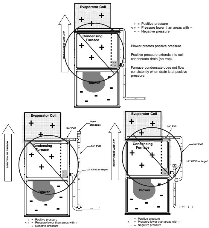
Fig. 13 – Example of Field Drain Attachment (Not Allowed) <sup>A14532</sup>
