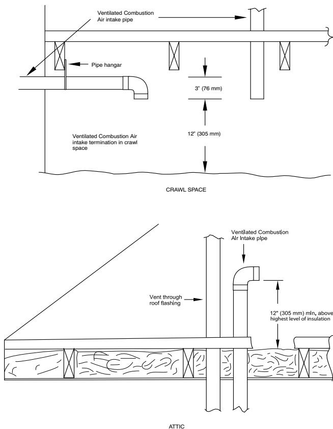
**Fig. 46 – Vent Terminations for Ventilated Combustion Air** A10497
