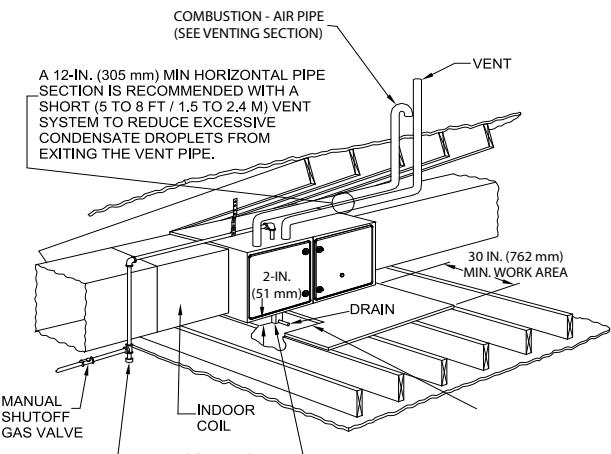
NOTE: FURNACE SHOWN AS DIRECT VENT APPLICATION. REFER TO THE VENTING SECTION FOR ALLOWABLE VENT CONFIGURATIONS
