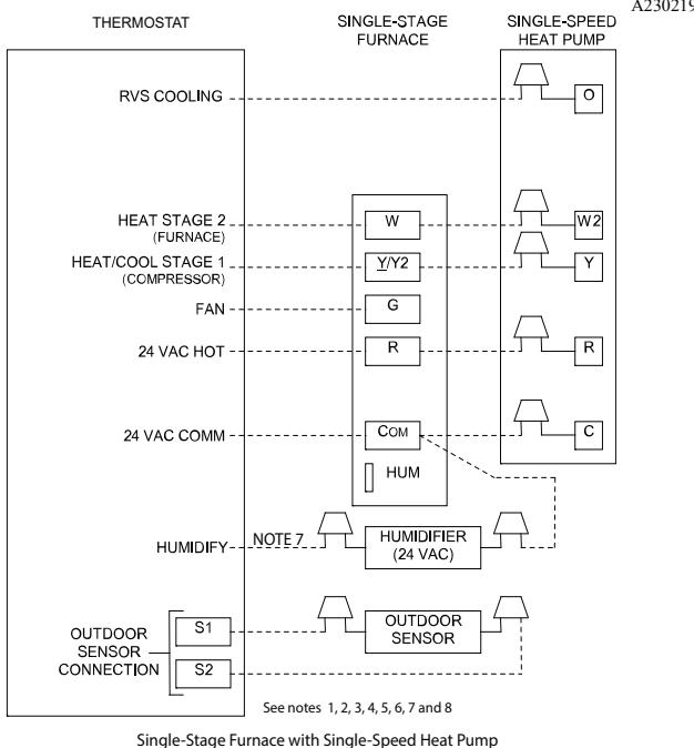
Single-Stage Furnace with Single-Speed Heat Pump
