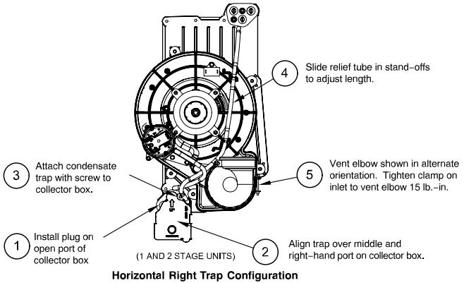
**Fig. 10 – Horizontal Right Trap Configuration**
