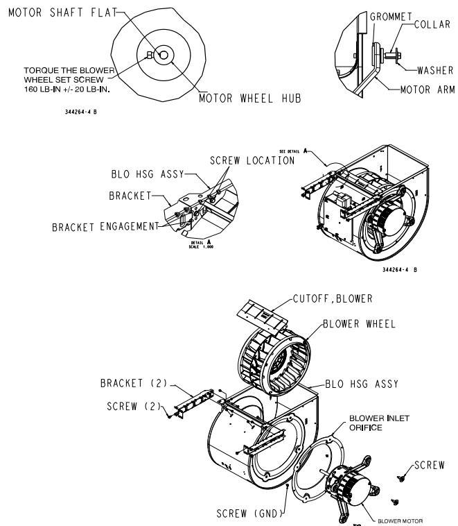
**Fig. 65 – Blower Assembly on 0401410 and 0401412** A190094B
