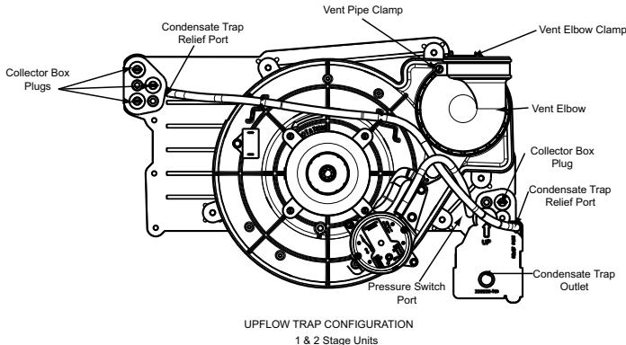
**Fig. 8 – Upflow Trap Configuration**
