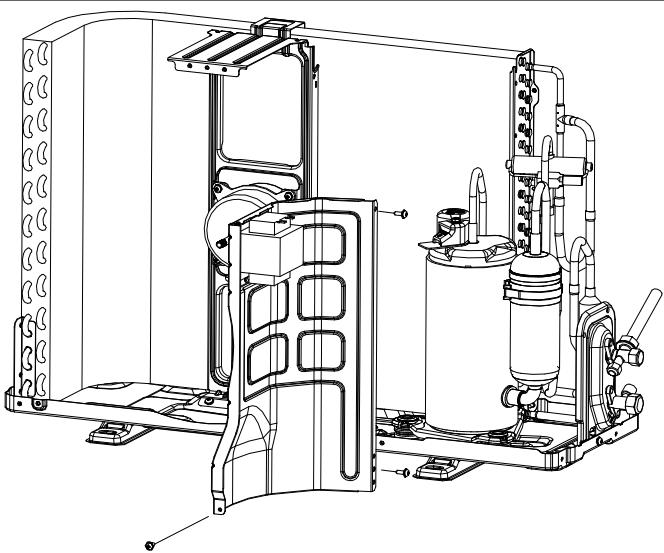
**8. Disassemble the 2-way and 3-way valve**
