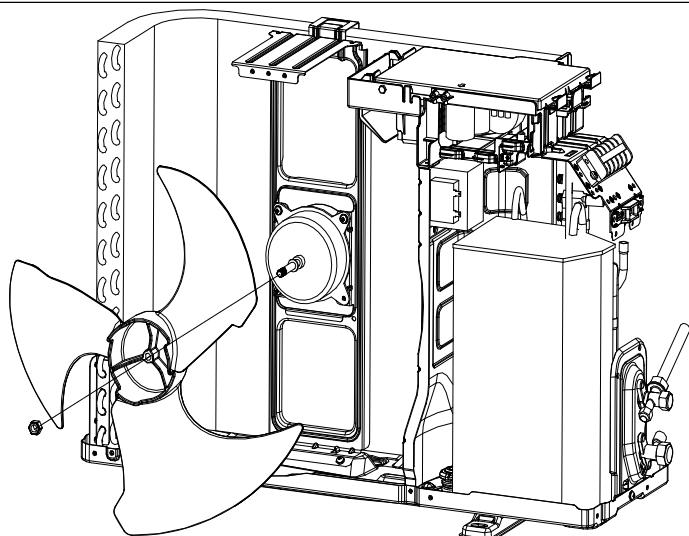
**5. Disassemble the electric box**
