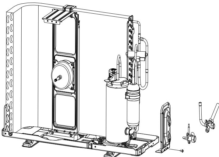
**9. Disassemble the 4-way valve assembly**
