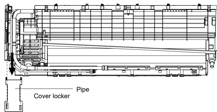
**8. Disassemble the evaporator**
