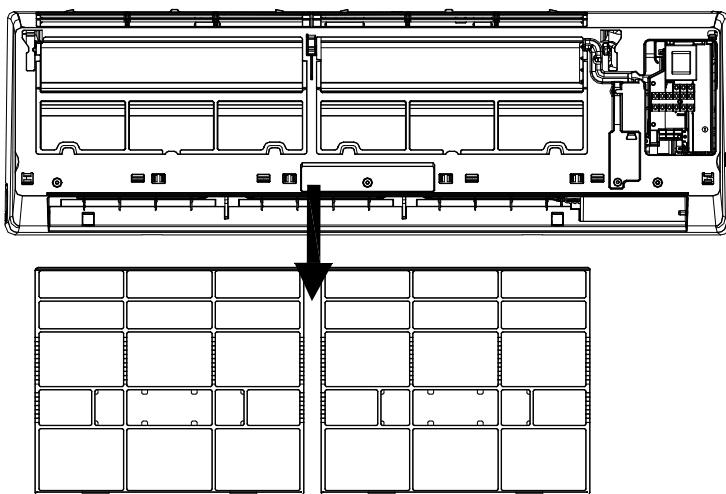
**5. Disassemble the middle frame**
